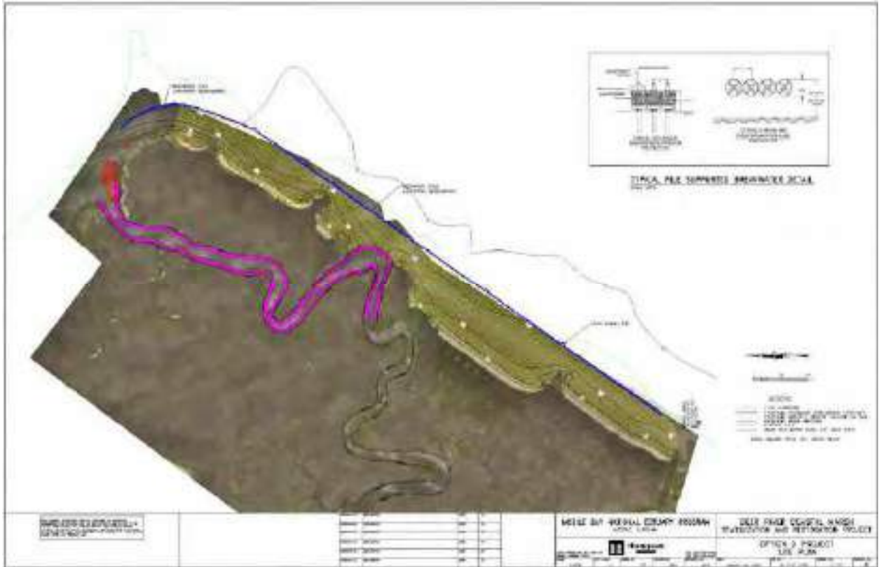
Figure 14: Alternative 3 – Pile-Supported Breakwater
